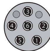
TV Pillow Speaker Interface Pinout
